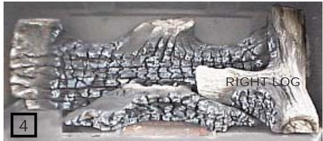
Tear the glowing embers into pieces and place onto the screen beneath the front log. Care should be taken to shred the embers into *thin, small irregular pieces* as only the exposed edges of the fibre hairs will glow when exposed to direct flame; however care should be taken to not block the burner ports. Blocked ports can cause an incorrect flame pattern, carbon deposits and delayed ignition.
