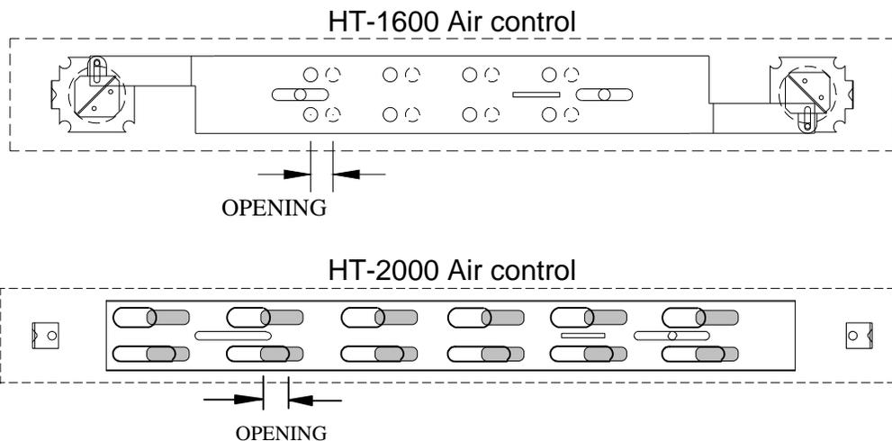
Please note that the HT series stoves do not have the same operating range. The HT-1600 type stove burned between 0.93 and 3.32 kg/hr during EPA testing. The 2000 serie achieved between 0.95 kg/h and 4.9 kg/h under the same conditions . Real operating conditions may give very different results than those obtained in the lab according to the species of wood used, its moisture content, the size and density of the pieces, the length of the chimney, altitude, outside temperature.
