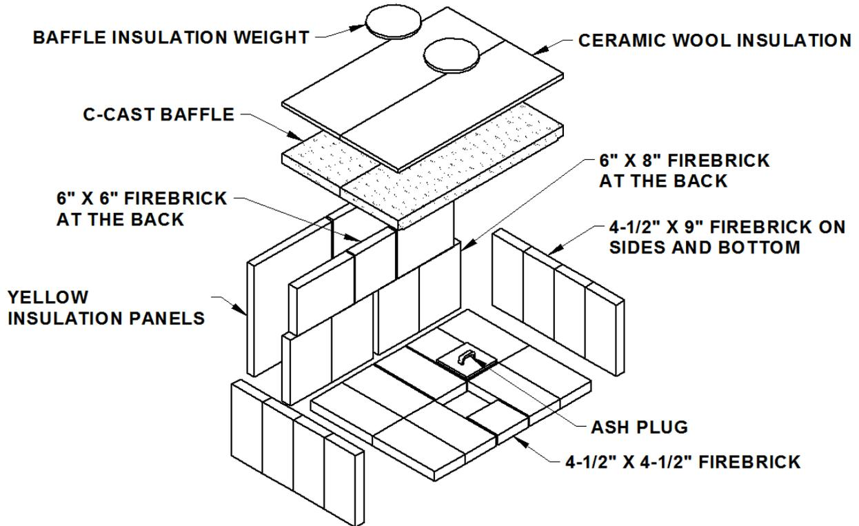
**Figure 3: HT-2000 Refractory Bricks Assembly**
