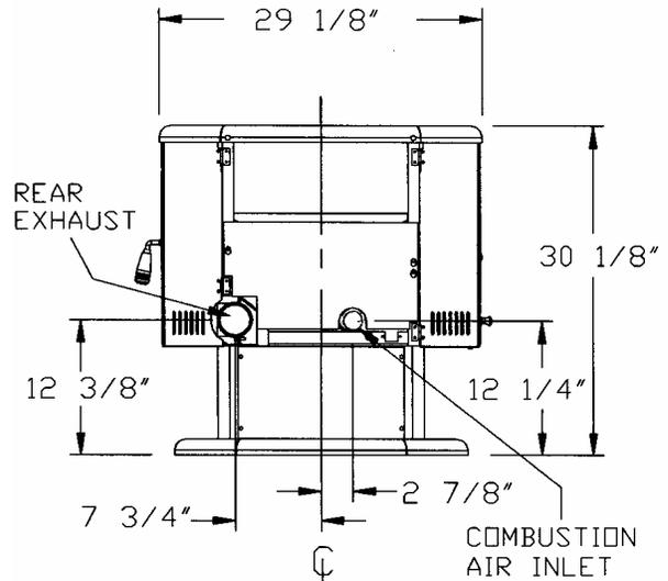
**REAR VIEW P2000FS****FIGURE 5**
