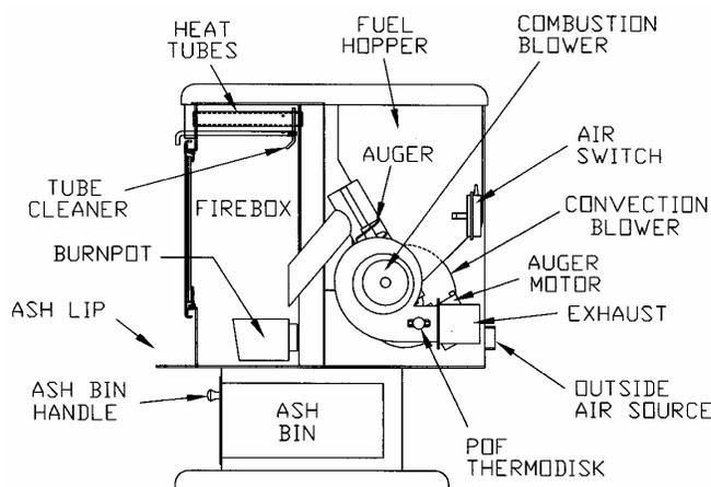
SIDE CUTAWAY – P2000FS
